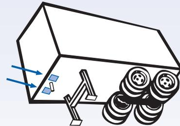
3. When the fifth wheel plate engages the trailer, the pouch ruptures to release the lubricant.
