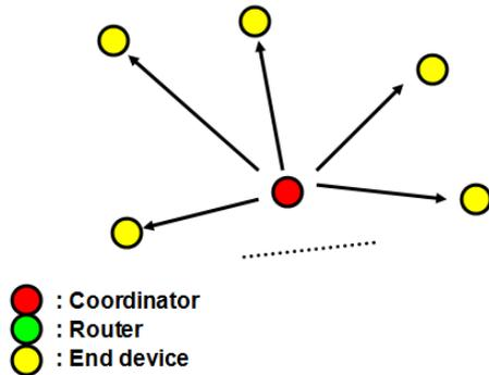
No Zigbee manager software necessary. Just power on the adapters with the same PAN ID and Channel no.. If you need to set multi network, please set the different PAN ID, channel no. and short address from section 8.3 and 8.5.
