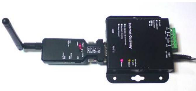
11.3 Virtual COM port via Internet: You can set the COM port via Internet. The controller will control the Zigbee mesh network remotely. Please contact us for more details.
