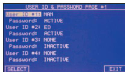
**User ID and Password** programmable for up to eight users, provides multiple levels of security and control, including alarm acknowledgement log by user
