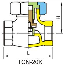
標稱壓力 Working pressure marking .....20 kgf/cm<sup>2</sup>
