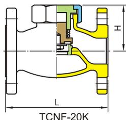
標稱壓力 Working pressure marking .....20 kgf/cm<sup>2</sup>
