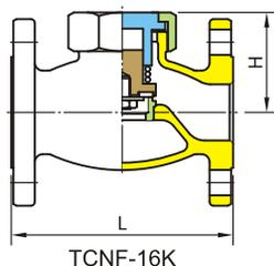
標稱壓力 Working pressure marking .....16 kgf/cm<sup>2</sup>
